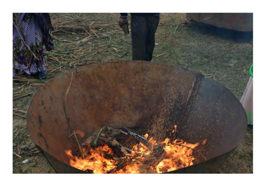
rice husks and sugar cane are excellent biochar feedstock when blended in the right proportion and timing with more bulky and energy rich feedstock like wood (needs experienced char maker!)
