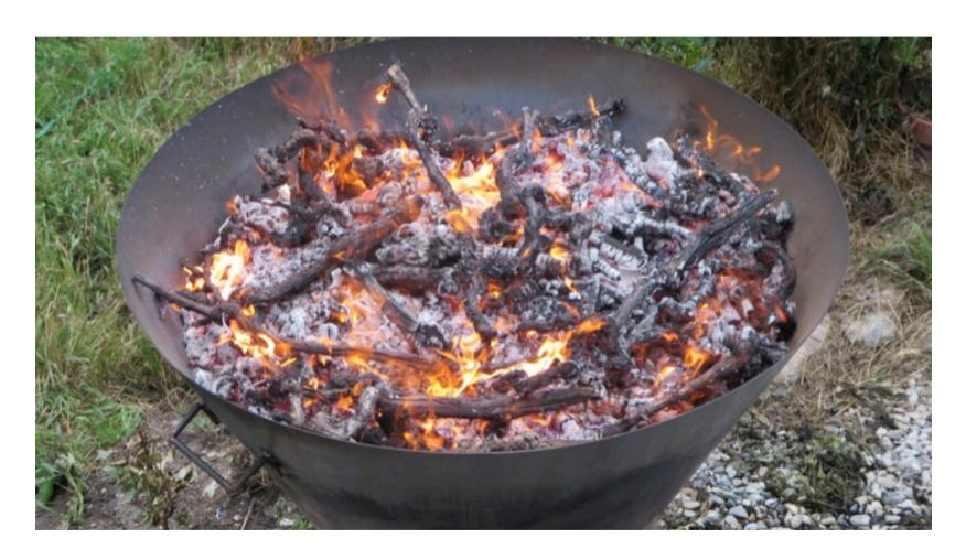
When ashes appear on the wood, put a next layer of wood. The charring continues beneath the fire front.
