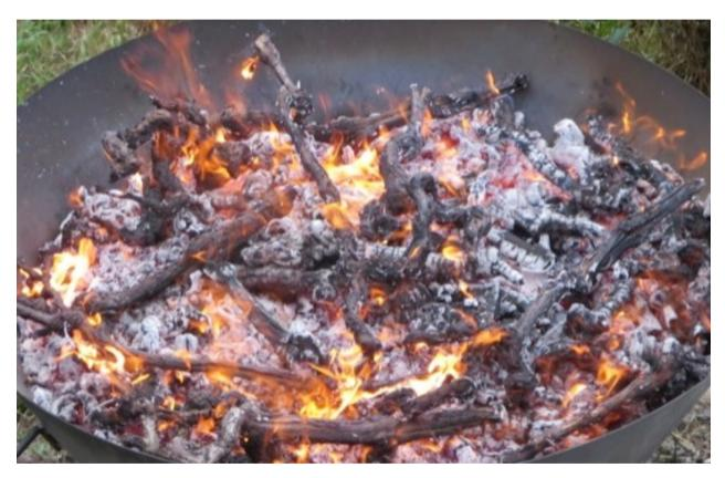
When ashes start to appear on the feedstock, put the next layer of feedstock. The charring continues beneath the fire front.
